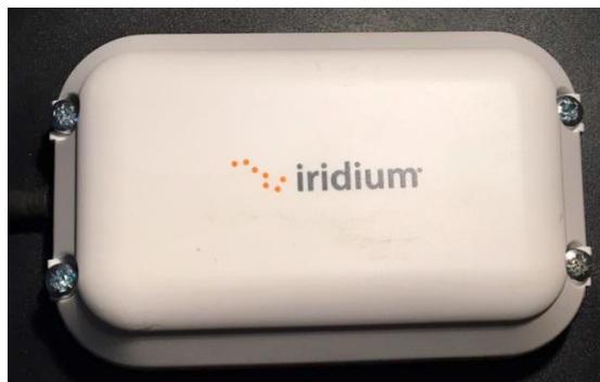
Figure 31: Screw Mount Installation
