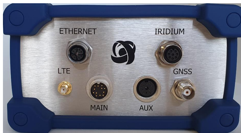
Figure 1: C-NavX1 GNSS Receiver Rear View
